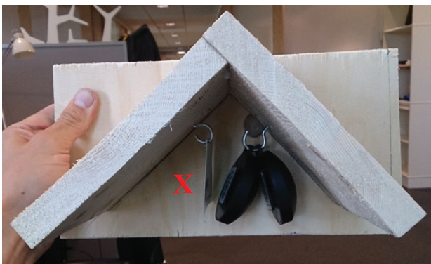
Fig. 2. Alpha track detector shelter used at each location. The TnP/RnP meshed and open detectors are not shown on photo but were mounted with clips, so that they were under the roof and in front of the back wall. Point of airflow measurement indicated by X.
