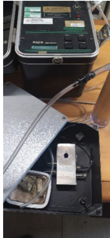
Fig. 8. Experimental setup with the prototype, the rock samples, and the tube of RAD7 inside the light-tight metal box.
